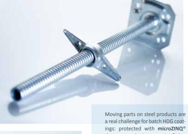
these parts obtain a superior fitting accuracy and remain movable after galvanizing due to the thin coating thickness and high viscosity of the microZINQ® alloy.
