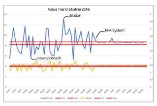
By synchronous measurement of up to three elements, in addition to pure coatings with copper, nickel, chrome and zinc, alloy coatings such as zinc-nickel, zinc-iron and cobalt-chrome can be optimally monitored. The very short analysis times of 2-5 minutes enable continuous compliance with the limit values and constant surface quality.
